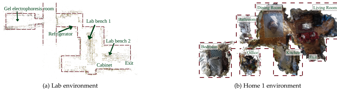
Fig. 2. Sparse SLAM points (2a) and offline dense reconstruction (2b) using [8] for two of our dataset environments.
